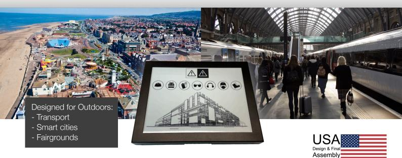
E Ink panels are used in displays that benefit from the unique features of ultra-low power consumption and visibility in both ambient light **as well as direct sunlight**. The Digital View 13.3" evaluation display is designed using E Ink e-paper display technology for outdoor sign applications benfitting from these unique features.
